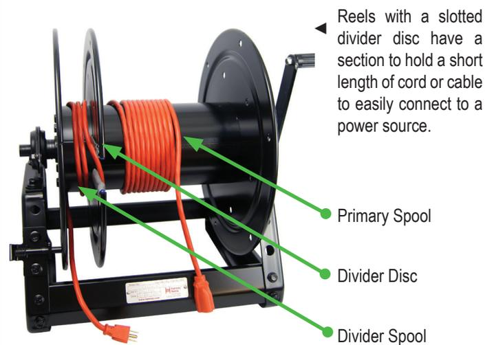
▶ Feed the desired length of cord or cable onto the small section from the inside of the reel through the slot in the middle disc, as shown.
