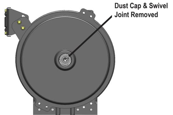
**FIGURE 2:** Dust cap and swivel (if present) removed.
