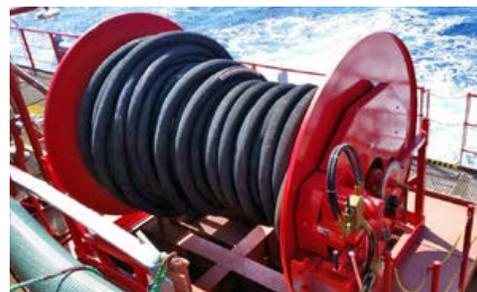
^ Hannay offers special marine grade finish or stainless steel construction to prevent rusting, rotting and corrosion – adding years to the life of every reel.
