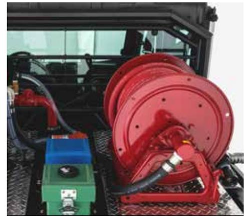
With a wide range of sizes and customizable features, Hannay reels are built to perform in a variety of situations. Pictured here is an 1800 Series reel holding 70 feet of ¾-inch booster hose.
