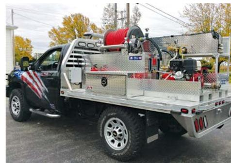
In addition to UTV side-by-side applications, KIMTEK fire/rescue skid units can also be fitted onto pickup truck beds.
