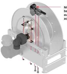
NOTE: If equipped it may be necessary to remove auxiliary rewind for access to bearing 3. Place split bearing bottom half on hub and rotate as shown in images, so bearing rests under the hub.
