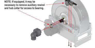
3. Remove mounting hardware holding bearing down and pry bearing top strap off using two flat head screwdrivers
