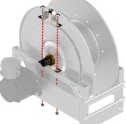
4. Lift joint side of reel and slide 1pc bearing off hub.
