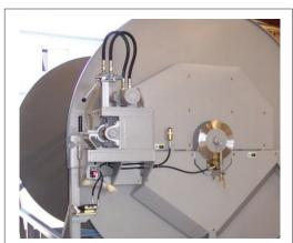
Figure 2: Image of Hydraulic Motor attached to a Hose Reel
