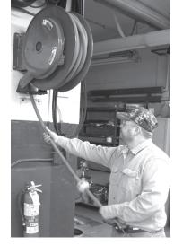
**NEVER REMOVE THE COVER CONTAINING THE SPRING.** Coiled springs are under tension and removal of cover can result in severe personal injury. Damaged spring motors should always be replaced.
