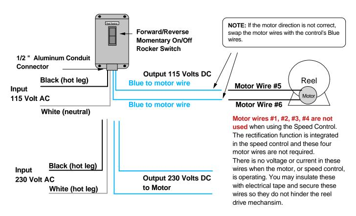
**Circuit Protection -** The installer must provide the 12 AWG, 2 conductor feed line and it must be on it's own circuit, protected by a 15 Amp circuit breaker in the electrical service panel. Do not use a ground fault breaker for the motor controller circuit protection.
