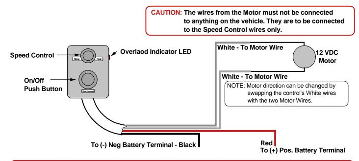
CAUTION: Do not connect the Black wire to the positive battery terminal and do not connect the Red wire to the negative battery terminal. This will cause a dead short condition across your battery terminals which will result in the circuit breaker tripping and will cause damage to the Speed / Switch Control unit. Do not use a motor direction, or reversing, switch on the Red and Black wires.
