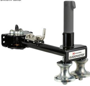
**Construction:** Grade 303 SST welded main body with black powder coat finish, wear-resistant Zamak 3 (zinc alloy) rollers and bearings on the top and bottom of the yolk with dust caps to limit dust and dirt intrusion. Switch has Class 1, Division 1 (Groups C & D) classification and is provided with a protective cover with push button switch.
