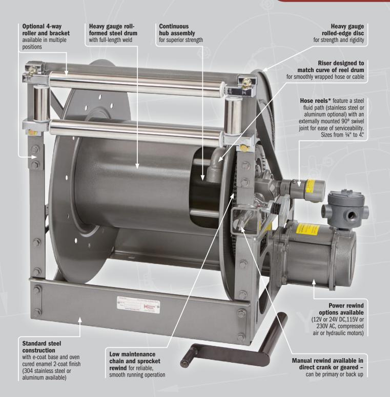
\*Cable reels feature externally mounted 3- or 4-conductor and 45-amp collector assembly for ease of serviceability; more conductors and other amperages available
