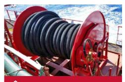
Hannay offers special marine grade finish or stainless steel construction to prevent rusting, rotting and corrosion – adding years to the life of every reel.
