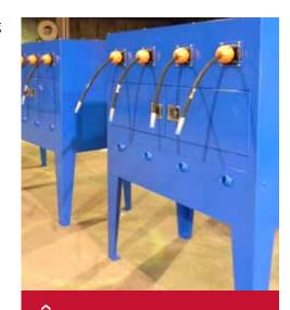
Each cabinet housed four different lubrication reels, which dispensed antifreeze, hydraulic oil, engine oil, and gear oil.
