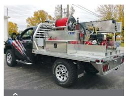
In addition to UTV side-by-side applications, KIMTEK fire/rescue skid units can also be fitted onto pickup truck beds.
