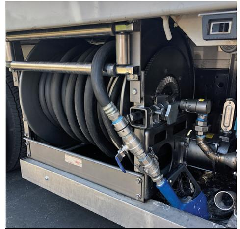
^ Hannay offers specially designed DEF fuel dispensing reels, built to handle both short and long hose lengths.
