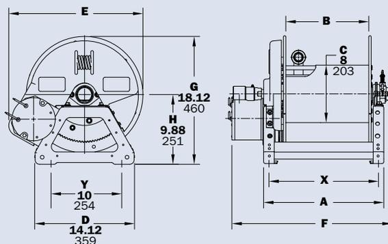
**AVISO:** A flexible connector must be used between the inlet pipe and the inlet swivel joint.
